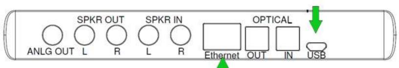
**Network** - The Condor connects to your local network, for control and setup purposes, but also for your SIP phone operations, through the RJ45 Ethernet connector
